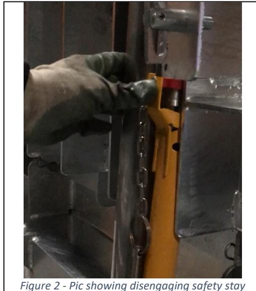
Figure 2 - Pic showing disengaging safety stay
