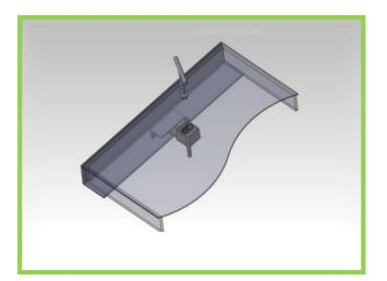
STEP 5 – When the key has been rotated a number of times the catch on the underside of the mechanism will become tight and move underneath the locking catch located on the frame. The access cover is now locked. Rotate the key so that it sits parallel with the slot and pull in an upward direction to remove key from the cover.
