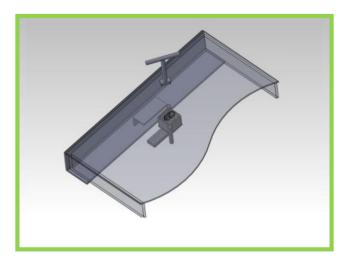
STEP 3 – When the key has been rotated a number of times the catch on the underside of the mechanism will become loose and move from underneath the locking catch located on the frame. The access cover can now be opened by turning the key 90° and pulling in an upward direction.
