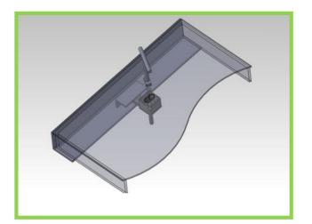
STEP 1 – Firstly ensure that you have the turnbuckle lock and lift key (COM0000741). Insert the supplied key in through the 38x18mm lifting slot in the top face of the cover and ensure it locates over the top of the turnbuckle bolt.
